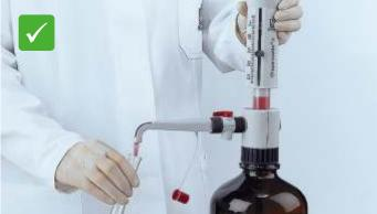
Dispensette®S has proven itself the world over with its wide range of practical applications reliable for accurate and safe dispensing even of aggressive reagents. It has been continuously improved over decades to meet the increasing demands of the laboratory.
