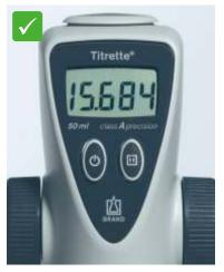
With the Titrette® bottle-top burette, you can titrate safely and reliably with the highest precision, even in close quarters, with no power hookup needed – in the lab, in production, or in the field.
