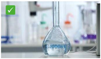
The safety coating helps contain the glass fragments in the event of breakage, and spillage of the medium can often be prevented.
